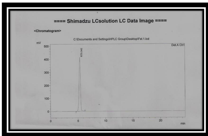
Figure 2: Typical chromatogram of Methyl 4-hydroxy benzoate (0.08mg/mL).
