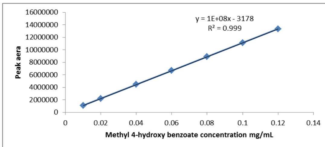
Figure 3: Calibration curve for Methyl 4-hydroxy benzoate.
