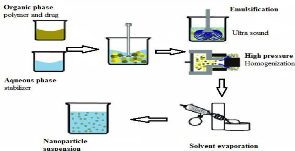
Fig. 2: Nanoparticle preparation using emulsion solvent evaporation methods.
