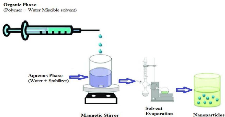
Fig. 3: Nanoparticle preparation using the solvent displacement method.
