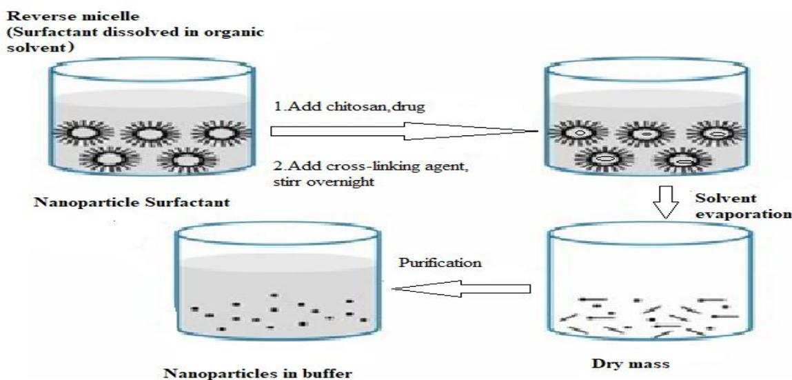
**Fig. 4: Nanoparticle preparations using salting-out method.**
