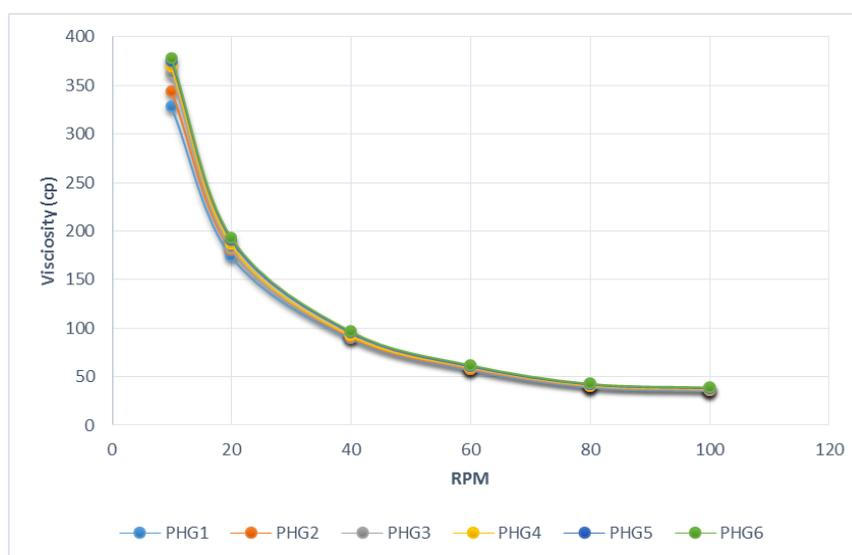
**Figure 3 Effect of shear on viscosity of gel.**
