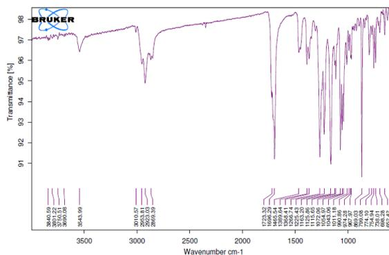
Fig. 7: FTIR spectra of optimized formulation.
