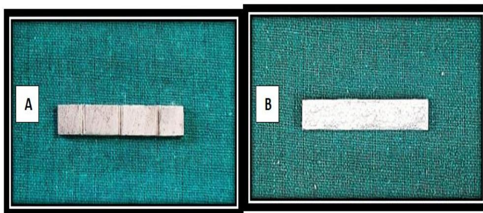
**Figure 1: Metal dies A) For dimensional accuracy and B) For flexural strength.**
