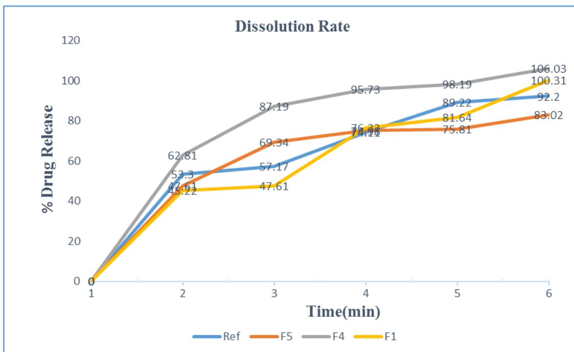
**Fig. 1: *In-Vitro* Dissolution Profile of Diclofenac Free Acid Formulations F1, F4, F5 and STD.**
