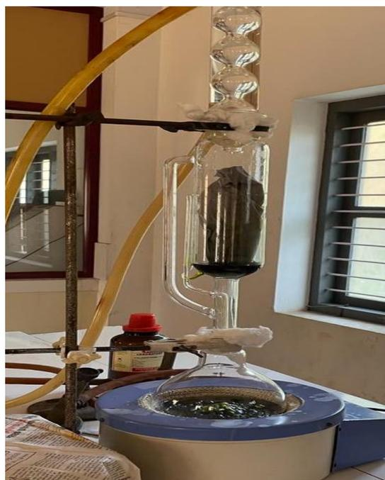
**Fig. No. 3: Soxhlet extraction.**
