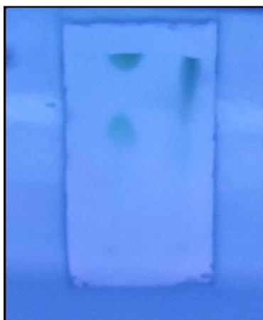
Fig. 1: TLC plate under UV light at 254nm.
