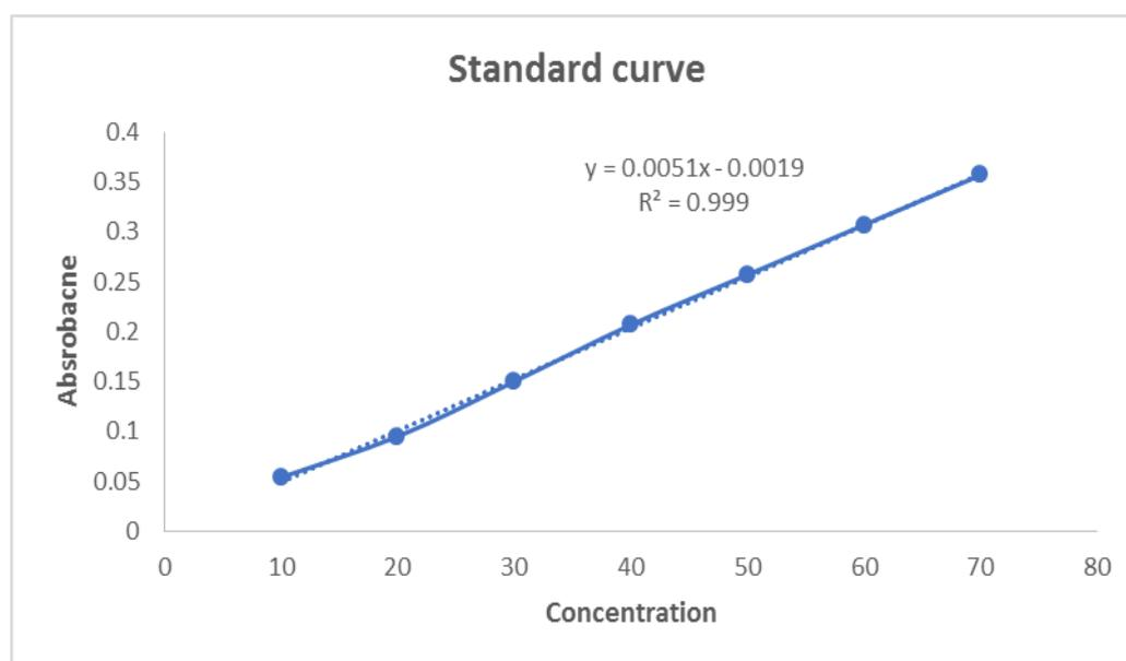
**Figure 2: Calibration Curve For Terbutaline.**
