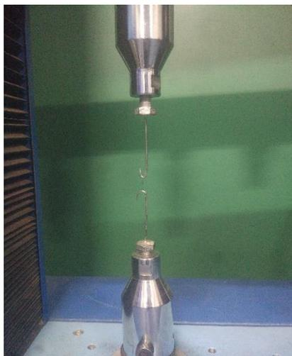
**Figure 2: The tensile strength was assessed using the Universal UltraTest machine (ACME Engineers, India. Model No. UNITEST-10)**
