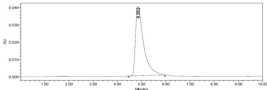
Fig-3: Chromatogram of Trazodone in Optimized Condition.
