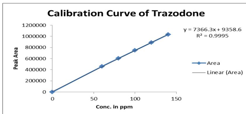
Fig-4: Calibration Curve of Trazodone.
