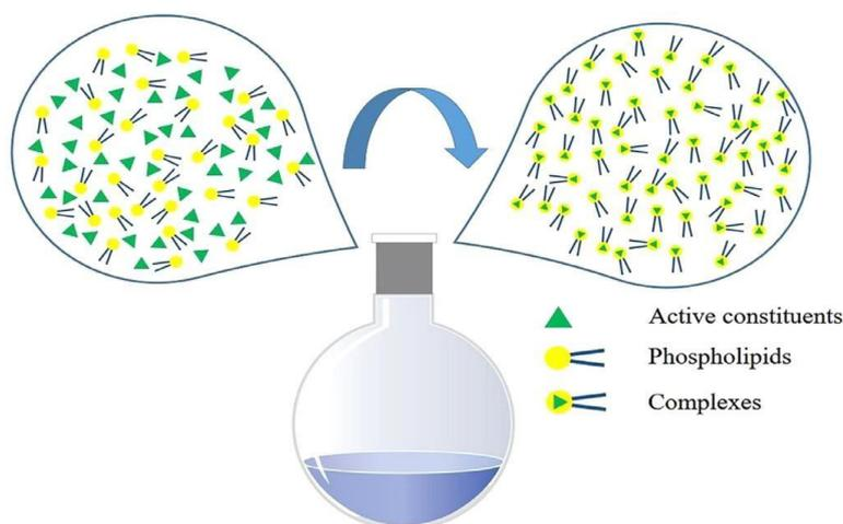
**Fig. 4:** Schematic representation of the preparation of phyto-phospholipid complexes by solvent evaporation method.<sup>[1]</sup>
