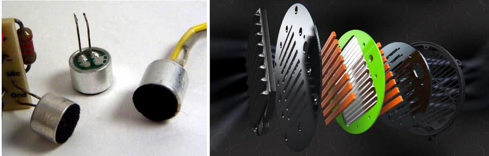
Figure-16: Electret and planar magnetic microphone.
