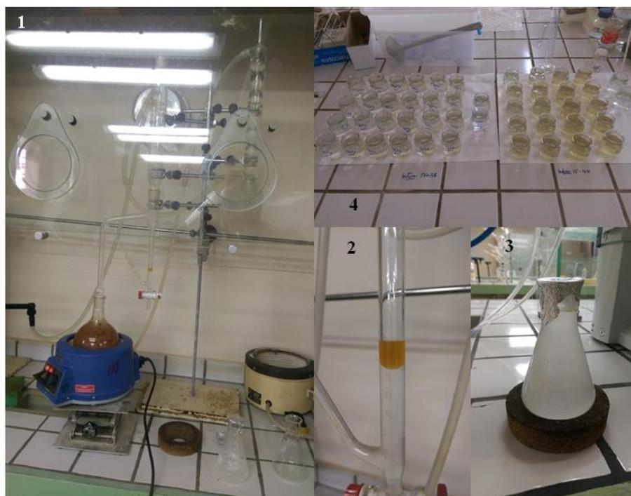
Figure 2: Production of plant extracts from the wood of *Tetraclinis articulata*; 1- extraction of essential oil by hydrodistillation using the clevenger; 2- Essential oil; 3- Floral water; Testing the toxicity effect of the wood of *T. articulata* on *Cx. pipiens* larvae from Mohammedia region.
