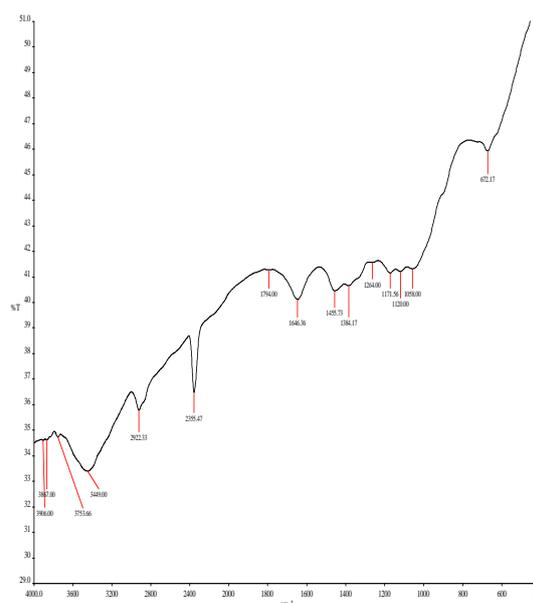
**Figure 4: FT-IR spectra of cellulose sugarcane bagasse. Figure 5: FT-IR spectra of cellulose corn cob.**
