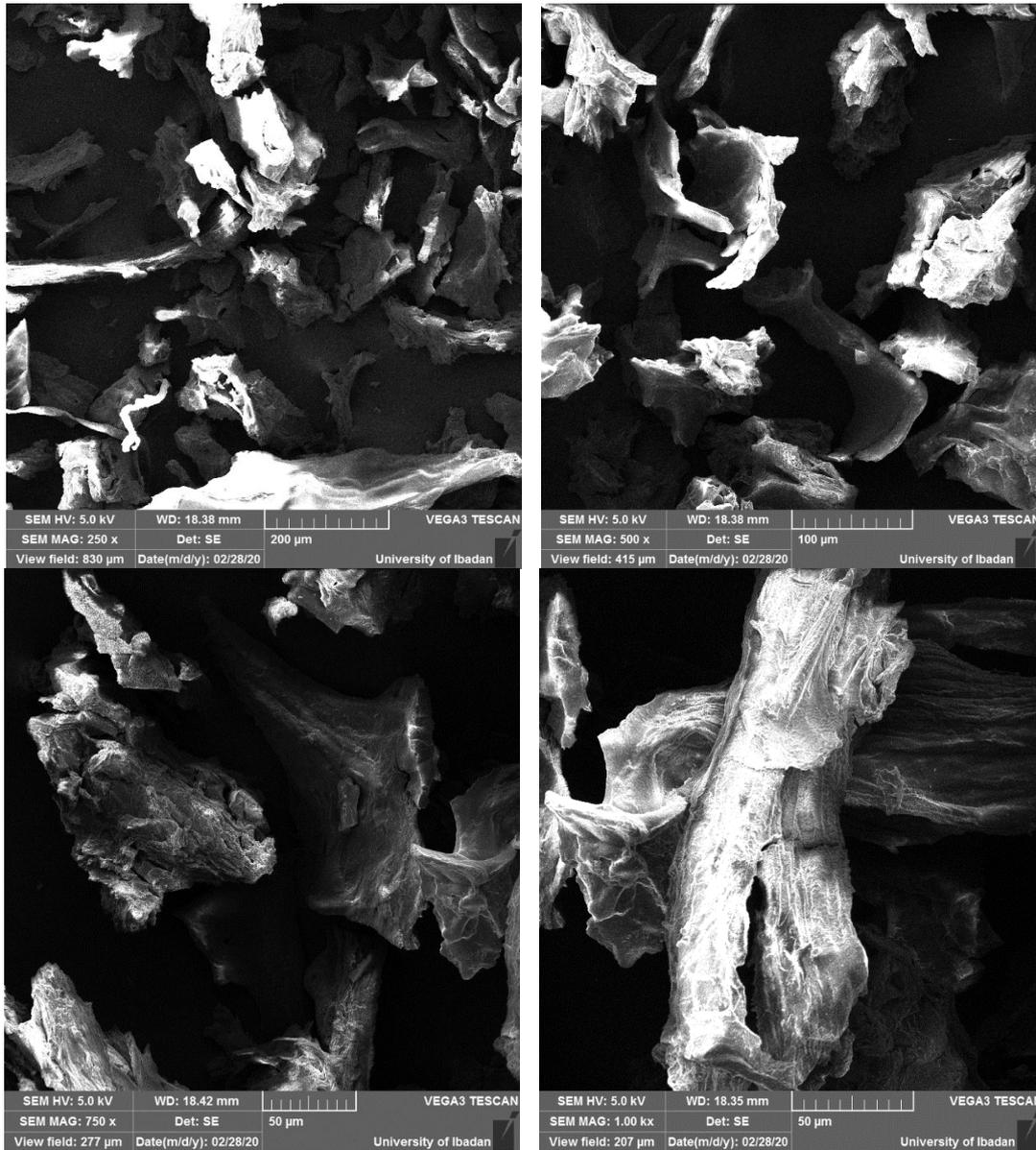
**Figure 6: Scanning Electron Micrographs of Sample A1, A2, A3 and A4 (Cellulose microparticles of Sugarcane Bagasse obtained using 60 % and 65 % Sulphuric acid for 45 minutes).**
