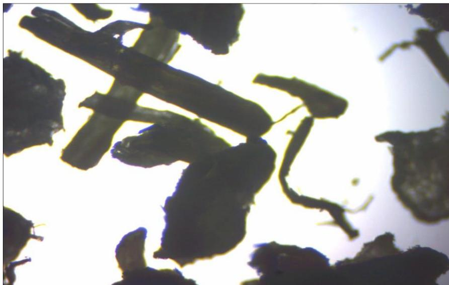
Figure 2: Photomicrograph of Sugarcane Bagasse Cellulose ( $\times 40$ ).
