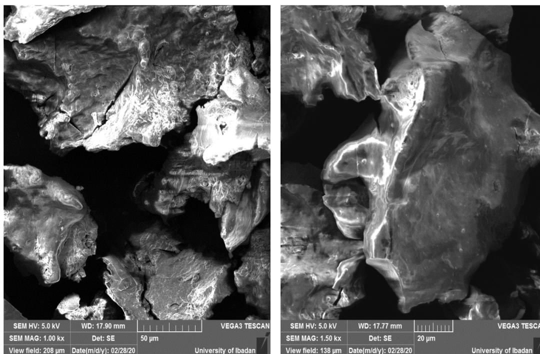
**Figure 7: Scanning Electron Micrographs of samples B1, B2, B3, and B4 (Cellulose microparticles of Corn cob obtained using 60 % and 65 % Sulphuric acid for 45 minutes) at varied magnifications.**
