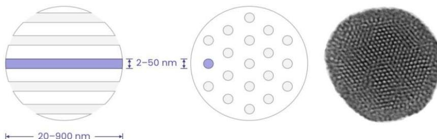
**Figure 1: Mesoporous silica nanoparticles.****Merits**
