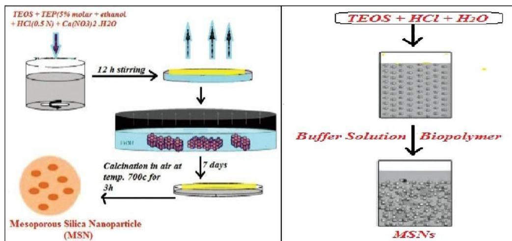
Figure 4: Synthesis of MSN'S by microemulsion method.
