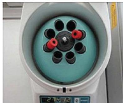
**Figure 3: A specific centrifuge with a motor turning at alternated and controlled speed from 2,400 to 2,700 rpm for 12 minutes.**
