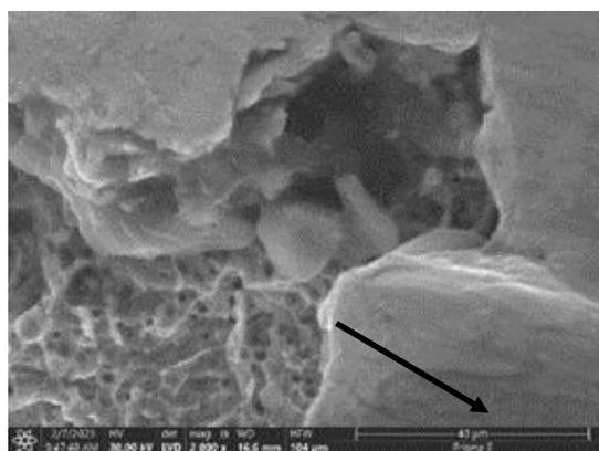
**Figure 5: SEM photomicrograph of a fractured surface of another W3-pro file in top view (x 3000) showing areas of elevations at the peripheries (black arrow).**
