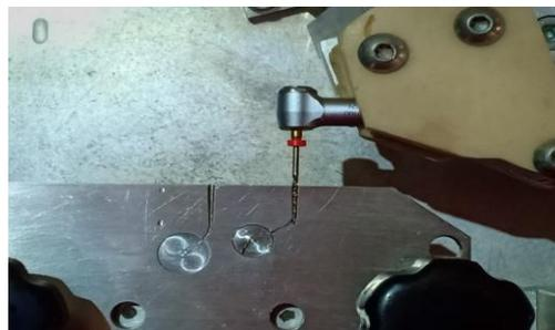
**Figure 1: File after fracture.**
