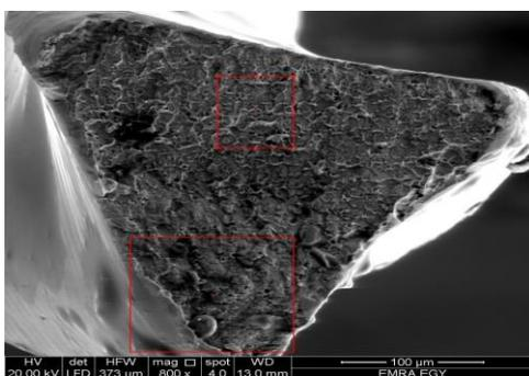
**Figure 2: SEM photomicrograph of a fractured surface of Revo-s file in top view (x 800) showing central fibrous appearance, areas of elevations at the periphery and dimples.**
