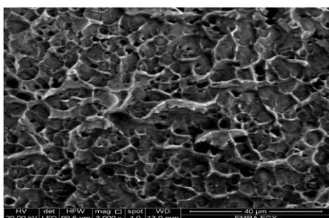
**Figure 3: Higher magnification of the same sample (x 3000), showing dimples, and central fibrous area.**
