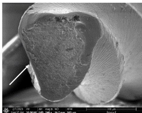
**Figure 4: SEM photomicrograph of a fractured surface of W3-pro file (x 800) showing cracks and microstructure voids (white arrow).**
