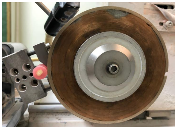
Figure 10: Mounting diamond disc 0.6mm thickness at speed 2500rpm.
