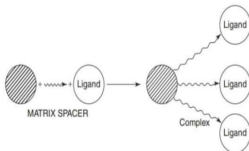
Attachment of the ligand to the matrix through spacer
