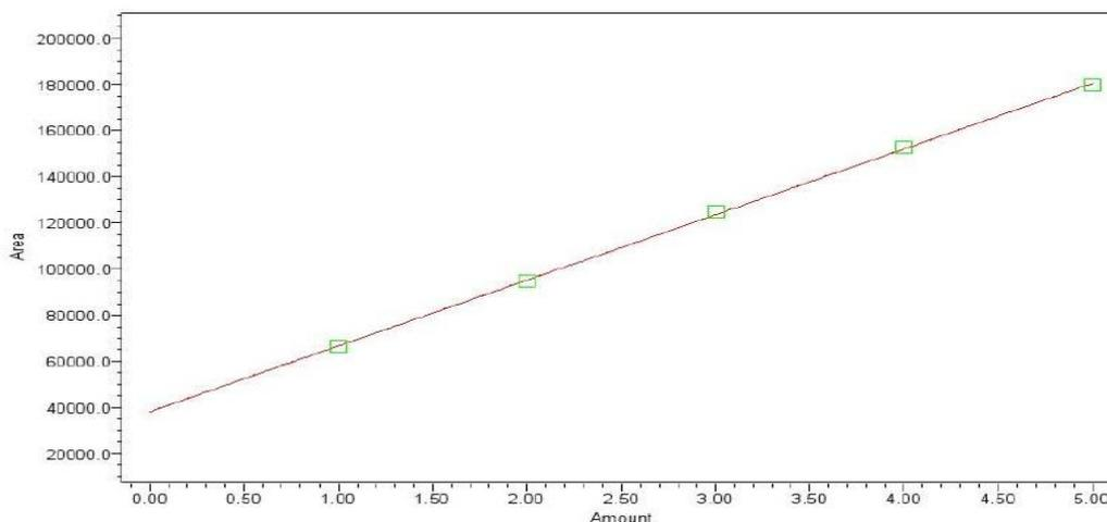
Figure 5: Calibration graph for Levamisole at 254 nm.
