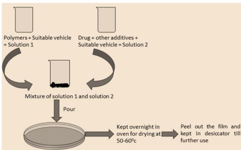
Fig. No. 2: Solvent casting method.
