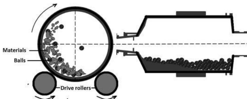
Fig. No. 5: Direct milling method.
