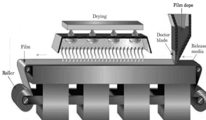
**Fig. No. 3: Solvent casting method.**
