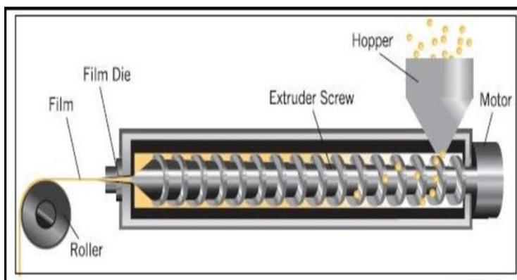
**Fig. No. 4: Hot melt extrusion technique.**
