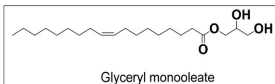
**Fig. 3: Molecular structure of Glyceryl monooleate.**<sup>[34]</sup>
