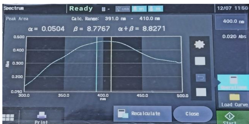
Figure 3: Shows the data interpreted by UV-Visible Spectro photometer which shows the highest absorbance from the range 391-410nm. Among this range at 399nm-406nm we observed the highest absorbance of 0.466.
