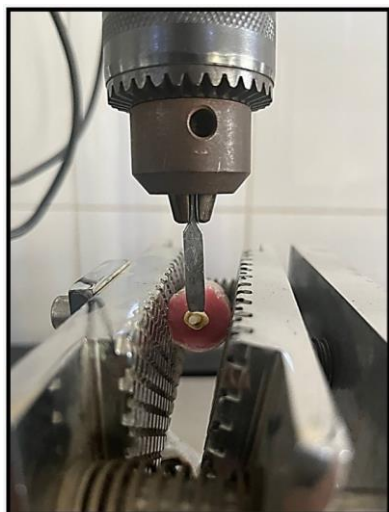
Shear Bond Strength Test in Universal Testing Machine
