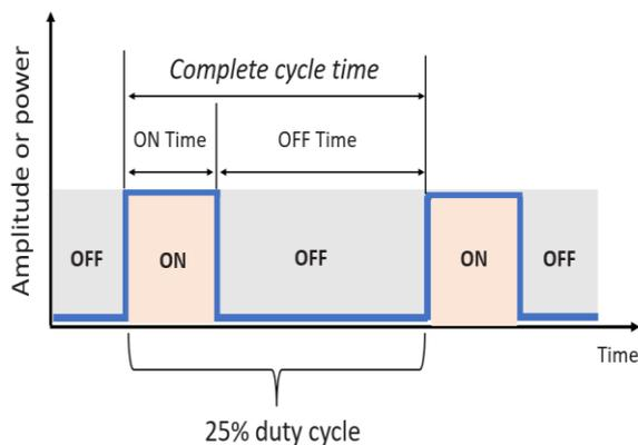
**Figure 4. Schematic showing the emitted pulses (ON) and the intervals between them where there is no laser emission (OFF), as well as the duty cycle.**
