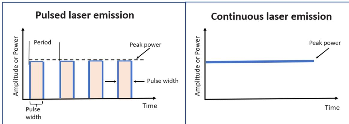
Figure 1. Schematic showing the structural differences of continuous and pulsed laser emission.
