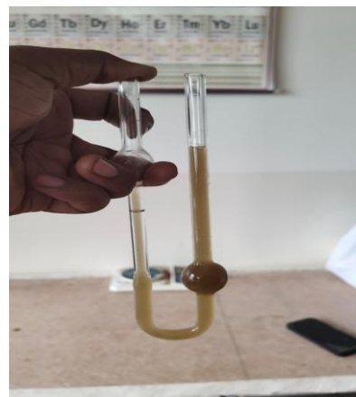
Figure No 14: Determination of viscosity by using an Ostwald viscometer.
