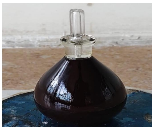
Figure 9: Determination of specific gravity using density bottle.
