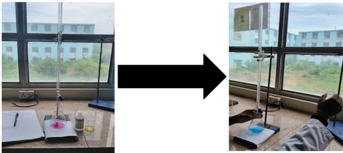
Figure 11: Determination of Acid value as a result the pink colour converted to blue colour when titrate with 0.1M KOH.
