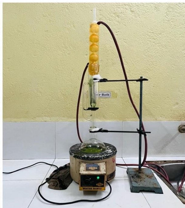
Figure 4.2 Crude extract of Leucas aspera leaves and Soxhlet extractor.
