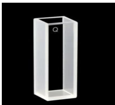
Fig. 5: Sample holder (Cuvette).
