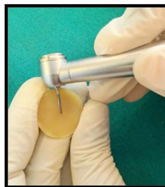
Fig. 6: Finishing of specimen with tungsten carbide bur.
