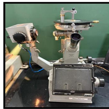
Fig. 10: Evaluation of microhardness done by Vicker's Hardness Testing Machine (Reichert, Germany).
