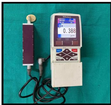
Fig. 9: Evaluation of surface roughness done by Profilometer (Surftest SJ-210) Mitutoyo, Japan,
