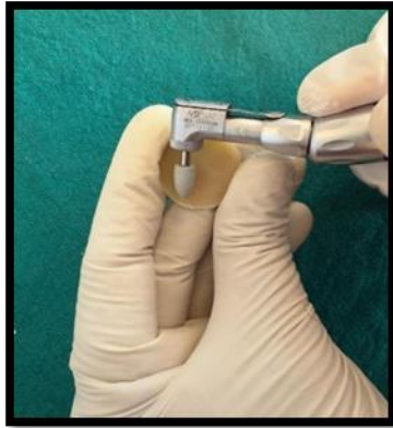
Fig.7: Polishing of specimens with Shofu One Gloss polishing kit.
