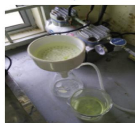
Aloe vera extract filtration using vacuum filter
