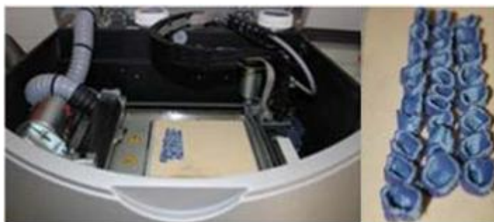
Fig. 1: Fabrication of Wax Patterns.
