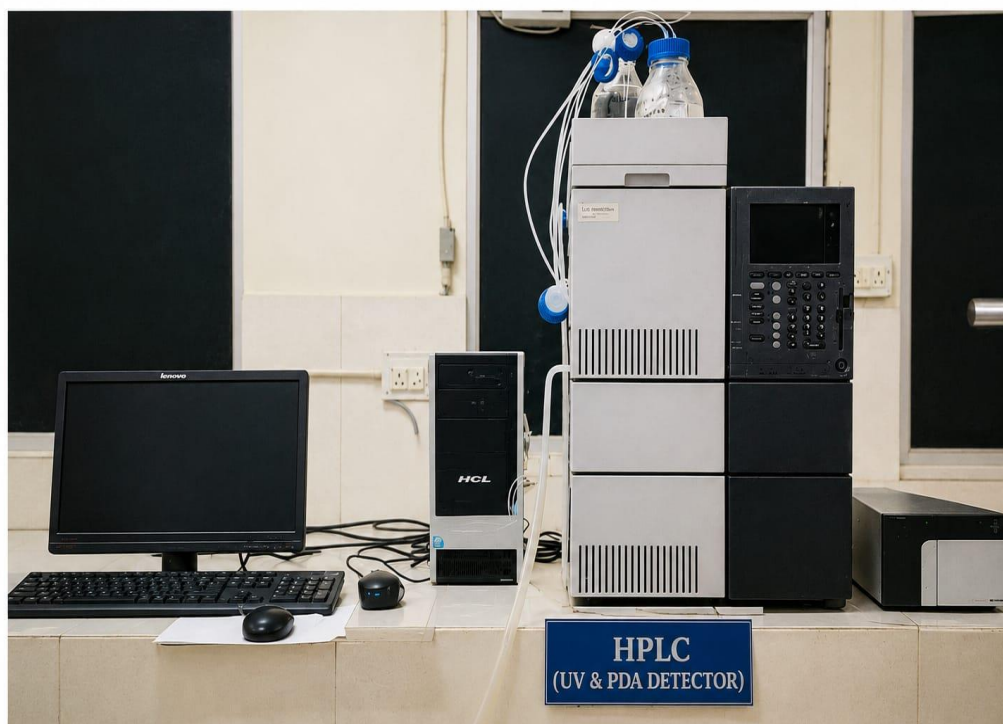
Figure 2. Instrumentation of High-Performance Liquid Chromatography (HPLC) System
