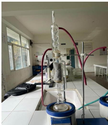
Fig. 3: Hot continuous extraction (Soxhlet).
