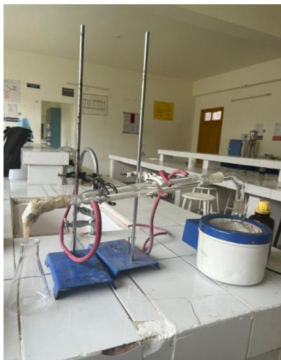
Fig. 4: Re distillation assembly
