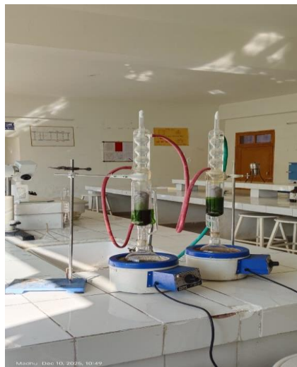
Fig. 2: Hot continuous extraction (Soxhlet).
