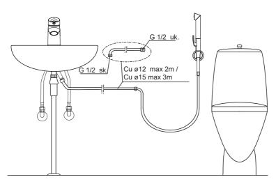
When using an extended Bidetta installation, Oras cannot guarantee the normal operation of the faucets. Bypass flow (water coming from the spout while using the Bidetta hand shower) may occur depending on the specifics of the installation.
