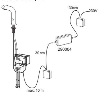
The transformer 290004 has 30 cm fixed cables on both sides for connection purposes.
