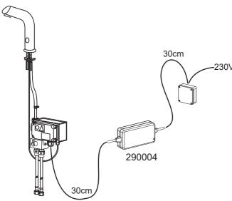
The transformer 290004 has 30 cm fixed cables on both sides for connection purposes.
