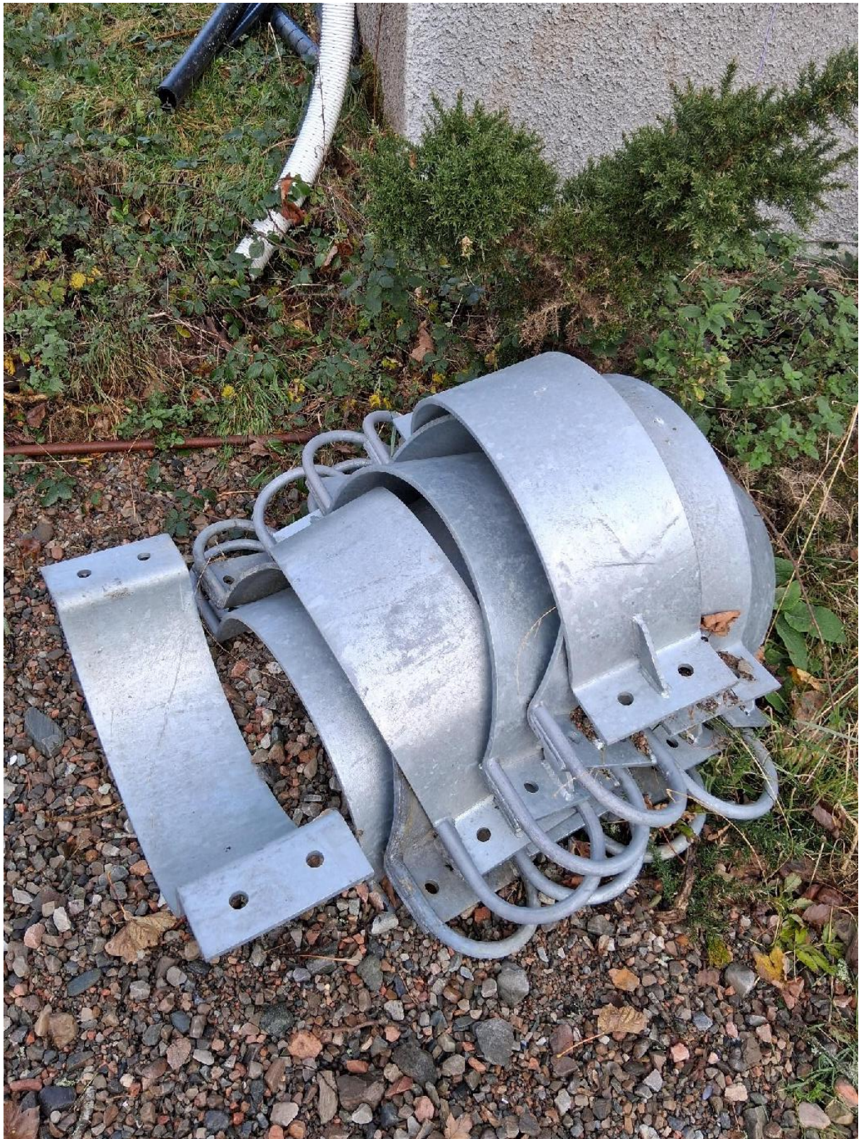
Photo 1: Clamps used to attach tidal barrier floatation tube to mooring chain. One of these clamps broke during the storm.
