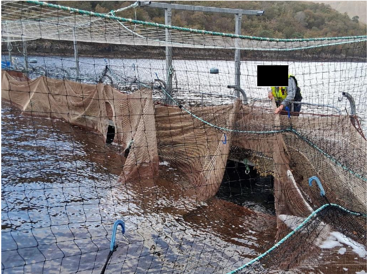
Photo 2: Holes in the net of cage 2. A member of site staff stands next to one of the larger holes
