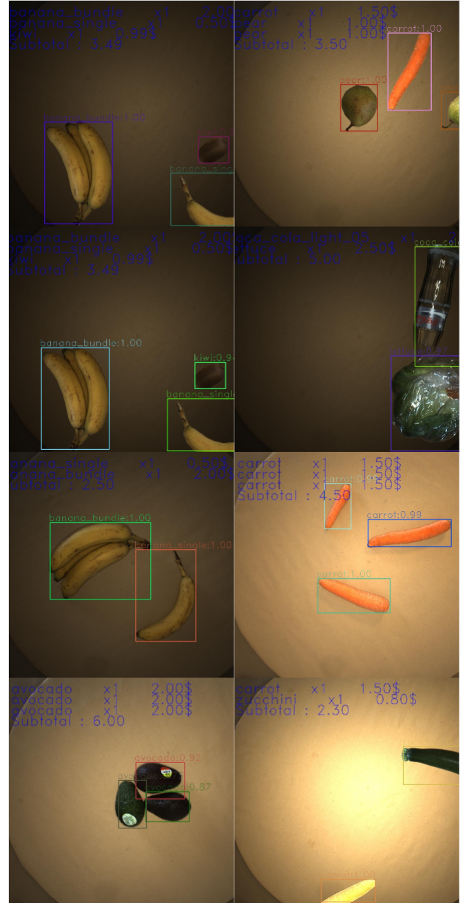
Fig. 6: Object Detection Prediction Model. The Name and Confidence Scores of each Item are Marked along with the Bounding Boxes. The Subtotal Information is Displayed at the Top Left Part of the Image.
