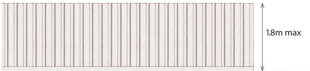
Fig. 4.4.2 - Interlot Fence Elevation
