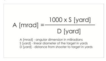
\*If the scoring target has more than one linear dimension (i.e. it is different from a circle or a square), than both the shortest and the longest diameter are used for calculation. The Stage Designer decides how many points will be awarded for scoring between those two values, according to the difficulty and specificity of the target.
