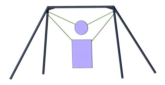
The metal plates for shooting distances up to 300 meters should be made from steel sheets with 16-20 mm thickness, in order for them to be relatively heavy enough, so that they don't roll or turn over, after a hit.
