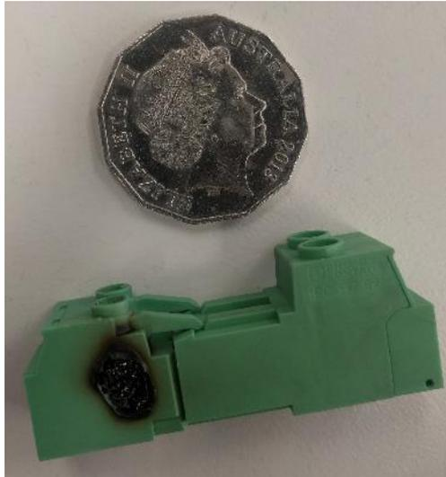
*Figure 14 Burnt out Tesla Powerwall 2 terminal block*
