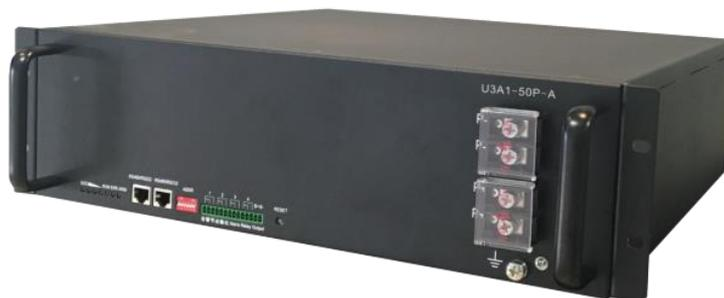
Figure 7. BYD B-Box battery module
