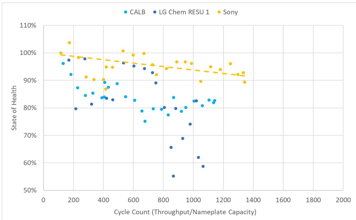
Figure 3 Average capacity fade results for Phase 1 Batteries
