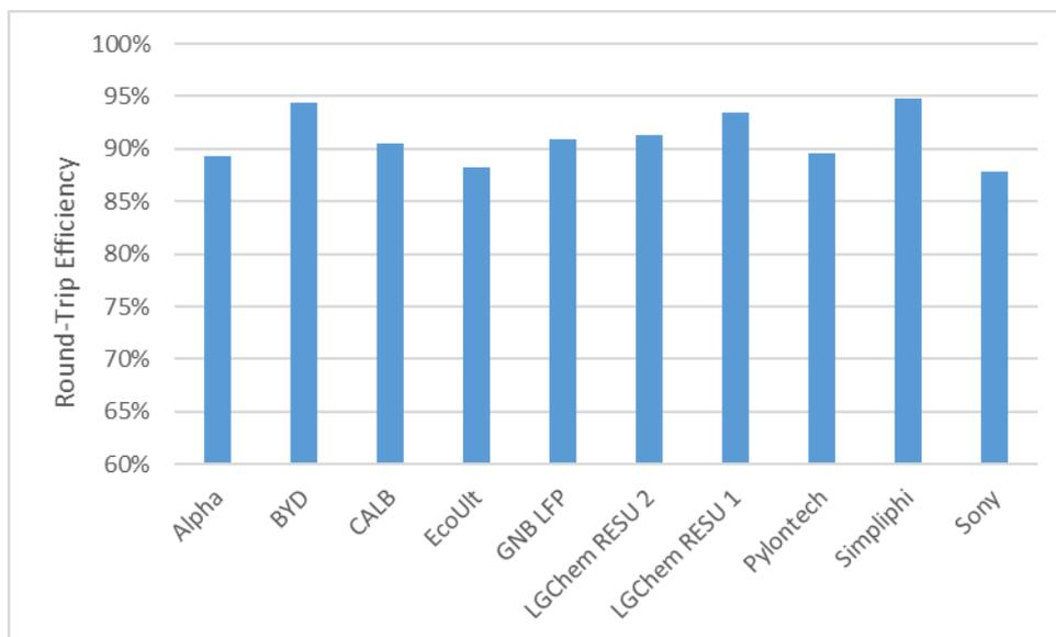
Figure 5. Average round-trip efficiency of various battery packs
