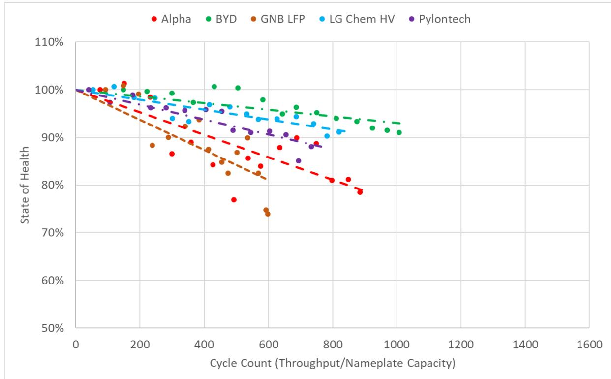
Figure 4 Average capacity fade results for Phase 2 Batteries
