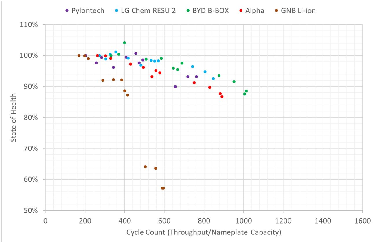
Figure 2. Capacity fade of Phase 2 battery packs
