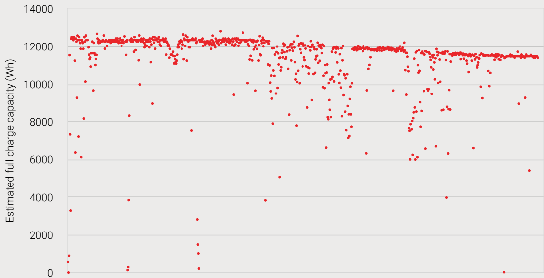
Figure 9: Estimated full charge capacity per cycle by the Tesla Powerwall 2 battery pack
