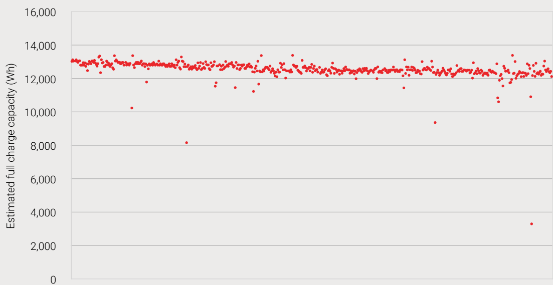
Figure 10: Estimated full charge capacity per cycle by the SolaX battery pack
