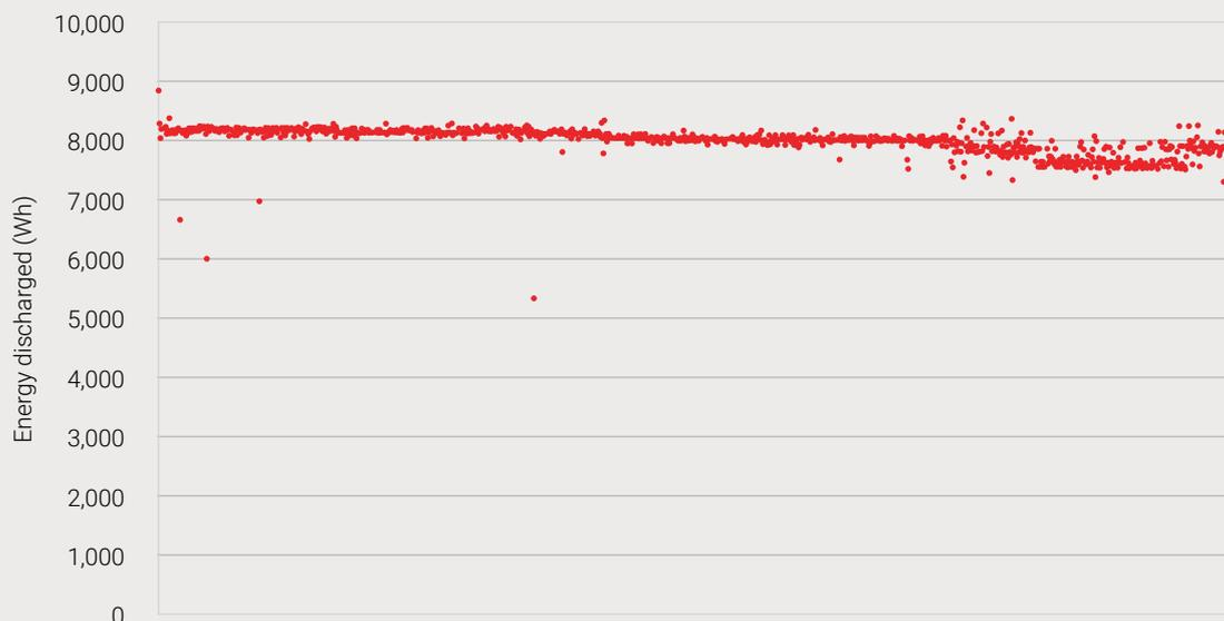
Figure 3: Estimated full charge capacity per cycle by the BYD LVS battery pack
