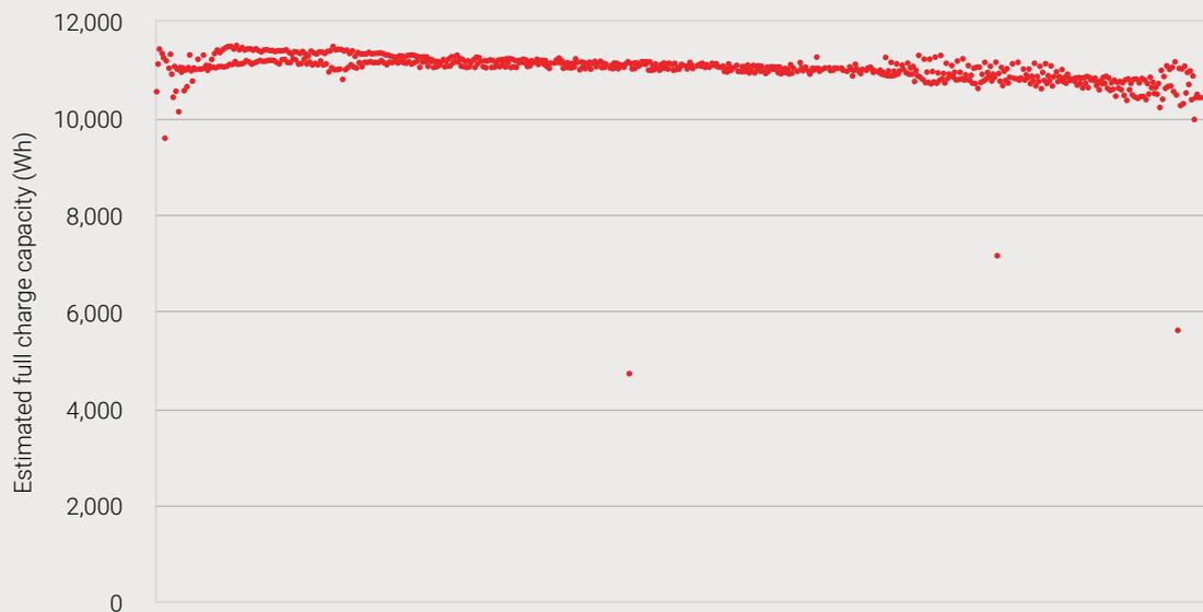
Figure 7: Estimated full charge capacity per cycle by the Redflow battery pack
