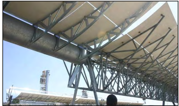
(d) Test loop for trough prototypes, SENER tough and ET I trough combined test system, Soler trough in background
