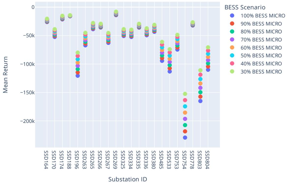
Figure 50: Effect of BESS cost on microgrid mean annual return
