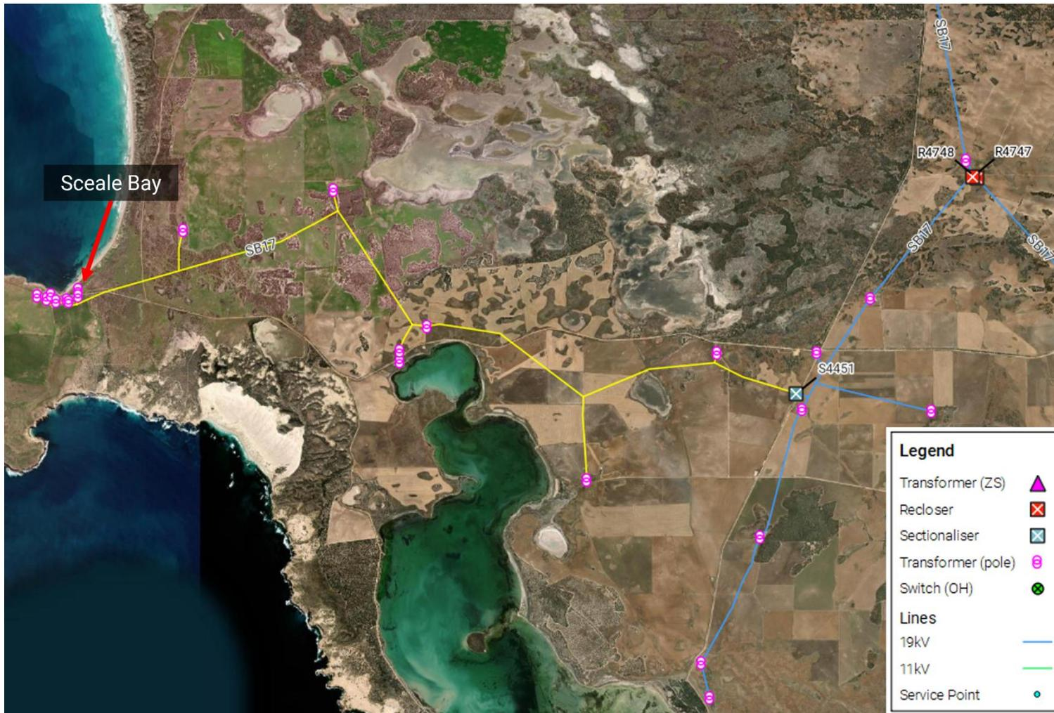
Figure 33: Proposed extent of the intermittent microgrid for Scele Bay (yellow)
