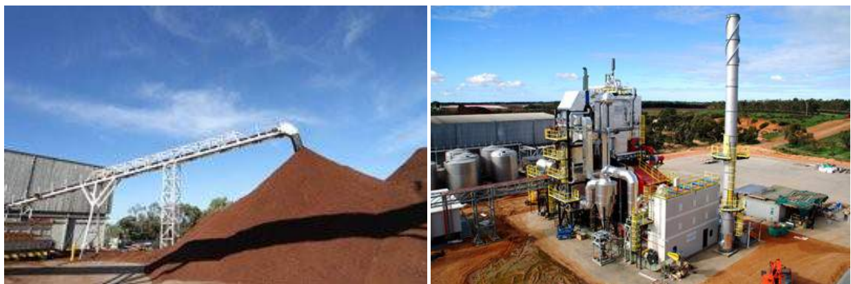
Figure 25: Automatic feed handling and 8MW th boiler using grape marc, photos Australian Tartaric Products
