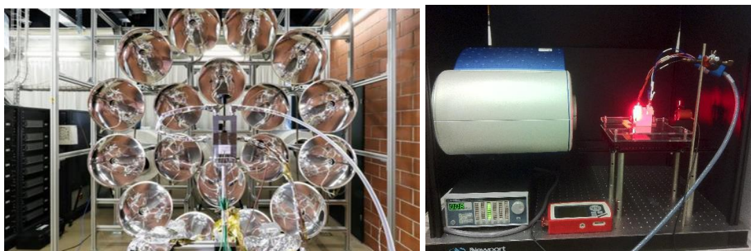
Figure 6: High-flux solar simulator test facility(left), LED 1 sun-simulator (right) at EPFL (source: https://lrese.epfl.ch ).
