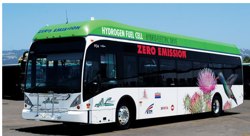
Figure 8: Hydrogen fuel cell electric bus tested by AC Transit in California in collaboration with NREL (source: NREL).
