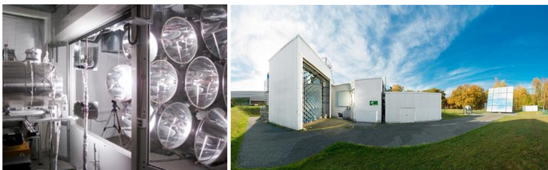
Figure 4: DLR high-flux solar simulator (left) and solar furnace (right) test facilities in Cologne (source: DLR).
